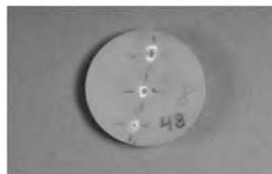
Figure 1: Root sections embedded in the acrylic disc with marking to Identify locations for hardness Measurement, sample no.48
